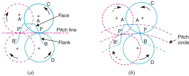
Fig. 12.7. Construction of cycloidal teeth of a gear.
