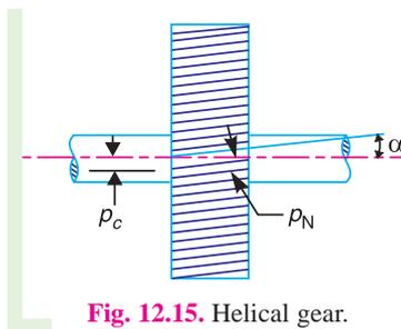
Fig. 12.15. Helical gear.
