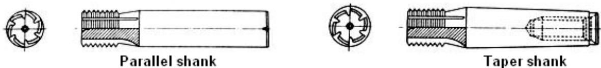
Fig. 2.49 Internal thread milling cutters
