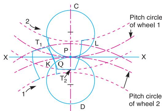
Fig. 12.8. Construction of two mating cycloidal teeth.
