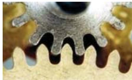
Let the wheel *A* be keyed to the rotating shaft and the wheel *B* to the shaft, to be rotated. A little consideration will show, that when the wheel *A* is rotated by a rotating shaft, it will rotate the wheel *B* in the opposite direction as shown in Fig. 12.1 (a).
