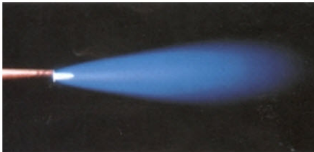
Figure 9.15 The neutral flame from an oxyacetylene torch, indicating temperatures achieved
